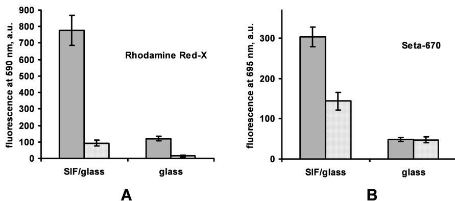
FIGURE 5. Examples of the gliadin assay using (A) Rhodamine or (B) Seta labeled Gli in the absence and presence of silver islands. Grey bars represent the signal in the presence of Gli and white bars represent the signal in the absence of Gli. The temperature was 22° C. The error bars represent the standard deviation calculated for the five different experiments.
